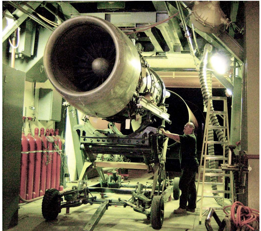
JT-8 Jet Engine Being Prepared for Test in KST Test Cell
