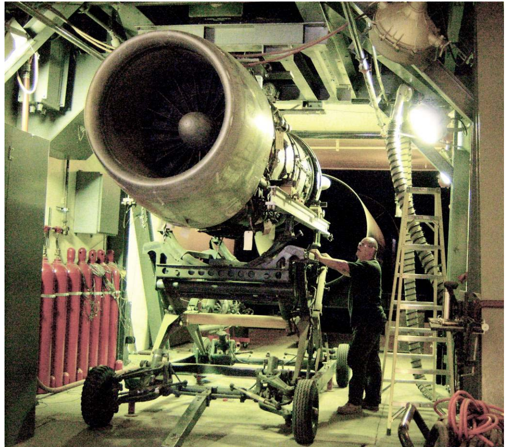
JT-8 Jet Engine Being Prepared for Test in KST Test Cell
